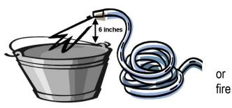
submerged in a source of contamination, the contaminant could be pulled back into the public water supply. This occurrence, known as backflow, can be prevented.
