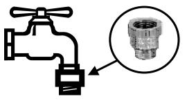
Another method of preventing backflow with a garden hose is using a device known as a vacuum breaker. Vacuum breakers are inexpensive devices that can be screwed onto your outside faucet. These devices will prevent contaminants from being siphoned back into your plumbing and the public water system.
